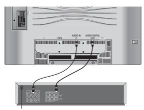
Select "Analogue" for "Sound transmission" for **analogue audio amplifiers**. The sound for the analogue amplifier is transmitted via the AUDIO OUT L/R connections of the TV to the audio amplifier. Connect the amplifier with two cinch cables. Specify under "Type of amplifier" whether the analogue amplifier is a stereo or surround amplifier.
